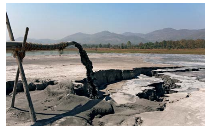
Waste from the second stage of bauxite processing is pumped from the Vedanta plant into a dumpsite which was previously agricultural land in Lanjigarh, Orissa.
